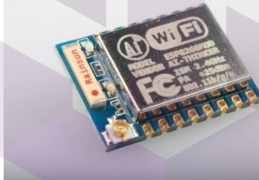
Figure 2 [Module Pin Counts, 16 pin, 16.0 mm x 21.2 mm x 3.0 mm]
